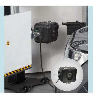
With VAS 701 001 the position of the VAS 6430 is permanently monitored during the calibration/adjustment of the ADAS. Changes in the travel axis or distances of the VAS 6430 to the vehicle are immediately displayed to the operator (optically & acoustically)
