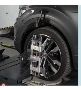
For the adjustment / calibration of assistance systems, only one additional camera on VAS 6430 (control camera) is necessary which can be used left or right to the direction of travel of the vehicle – measuring procedure is faster, allowing operators to measure more vehicles per day.
